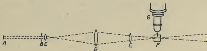
A. Arc Lamp. B. Slit. C. Primary Lens. D. Secondary Lens. E. Condenser (in. objective). F. Cuvette. G. Microscope.
